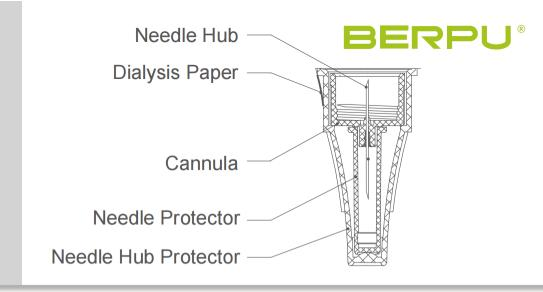
29G to 34G needle length from 4mm to 13mm
